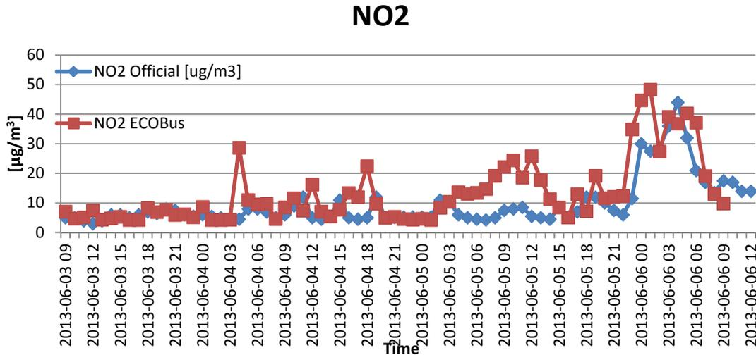
Figure 9: comparison of official and EcoBus NO<sub>2</sub> measurements
