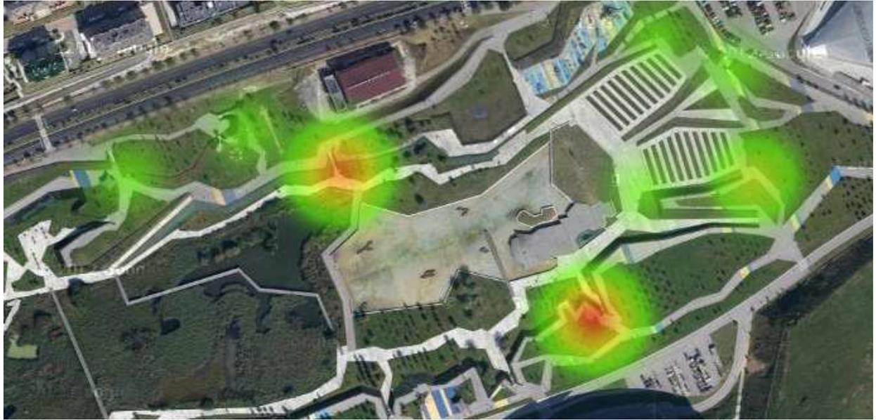
*Figure 31. Heatmap based on the SoilMoisture tension measurements carried out in Las Llamas park*
