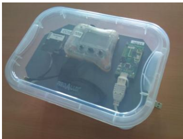
Figure 3: UZL cluster with an iSense, Pacemate and TelosB mote
